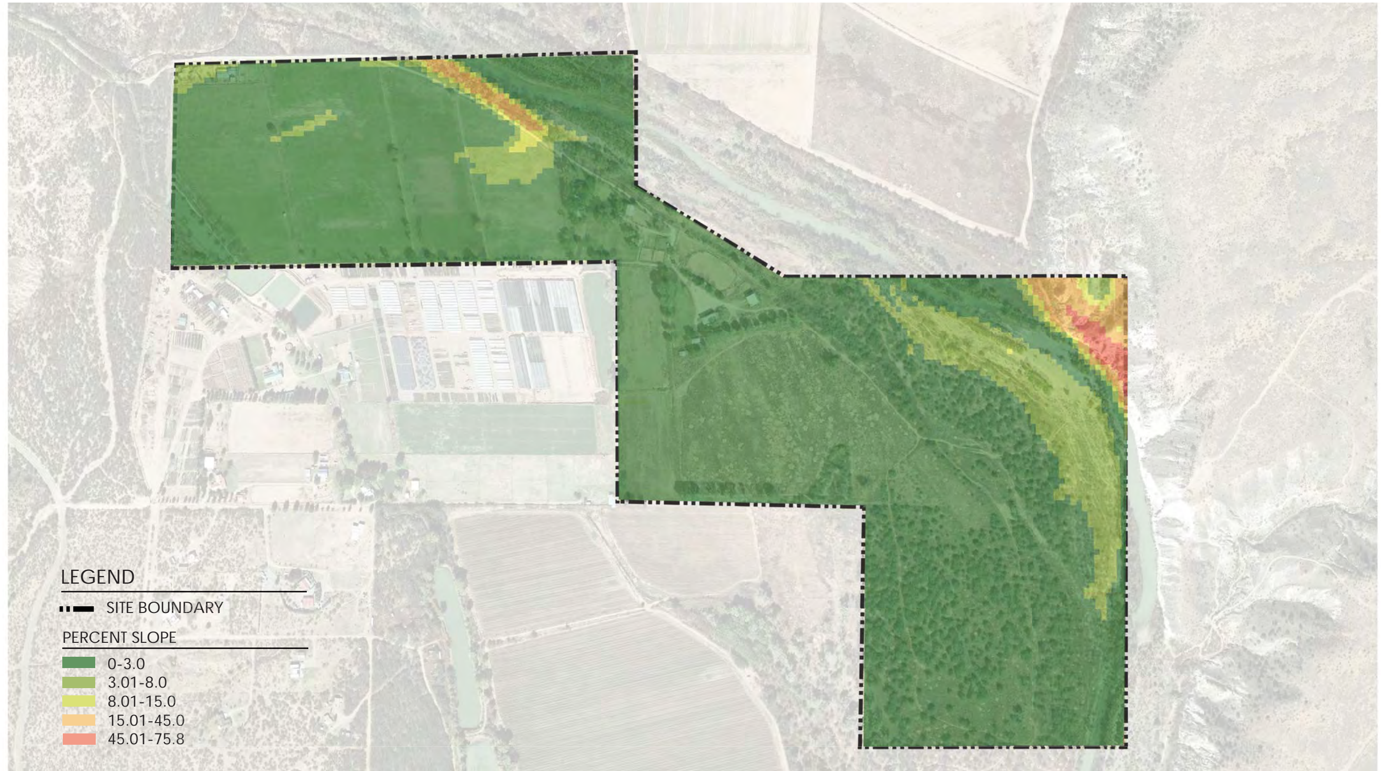
FIGURE A-6, SLOPE ANALYSIS
